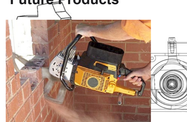
Gasoline Powered wood + Brick + Mortar Saw
